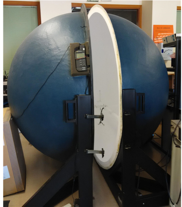
Fig. 17. Integrating sphere and spectrophotometer from LabSphere Inc. used for the measurements.
