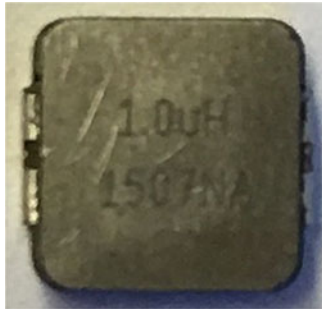
Fig. 15. Picture of the selected metal powder composite inductor for plastic packaging.
