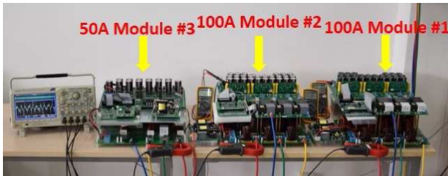
Fig. 15. Hybrid modular three-level SAPF prototype.
