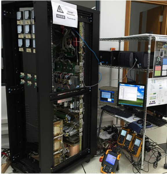
Fig. 13. Experimental setup of the 110 V-10 A HGCI experimental prototype.
