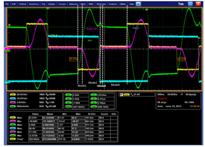
Fig. 32. Experimental results: CH1-Yellow: V_p ; CH2-Blue: V_{ds} of FET D; CH3-Pink: V_{p,sec} ; CH4-Green: -i_{res,prim} ; i_{res,prim} peak = 2.54 A, reflected i_{res,sec} peak = 17.8 A, i_{park} = 10.5 A, f_{sw} = 386 kHz, I_o = 25 A.
