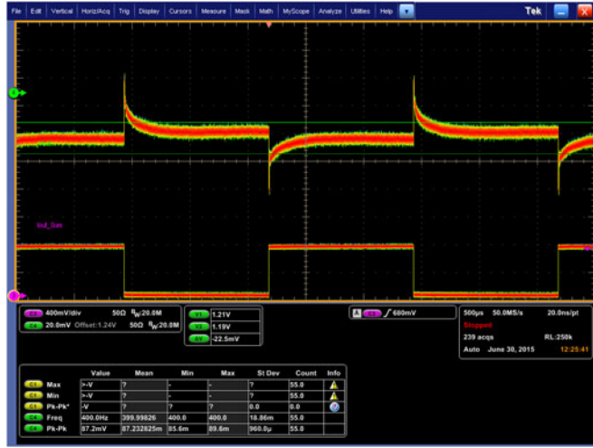
Fig. 39. Load transient performance at 400 Hz switching, 0–25 A, 12.5 A/ \mu s (CH3-Pink: current reporting signal for the load tester, 15 mV/A; CH4-Green: Output Voltage with 20 MHz BW).
