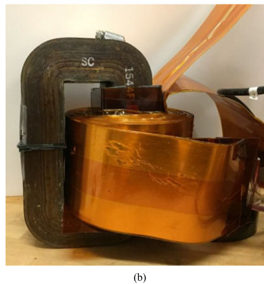
Fig. 10. Fabricated hybrid transformer: (a) magnetic core and permanent magnets and (b) final fabricated hybrid transformer.
