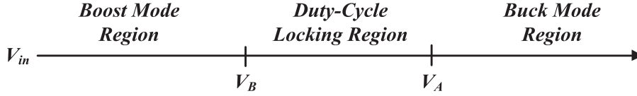
Fig. 7. Relationship between mode operation and input voltage.
