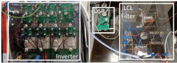
Fig. 10. Single-phase grid-connected inverter with PLL—experimental setup.
