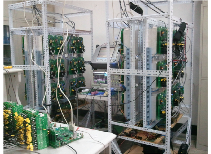
Fig. 14. Three-phase back-to-back MMC prototype.
