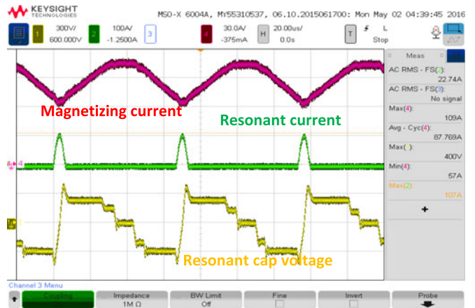
Fig. 20. Zoomed-in cycle-to-cycle waveforms for magnetizing current, resonant capacitor voltage, and resonant inductor current.
