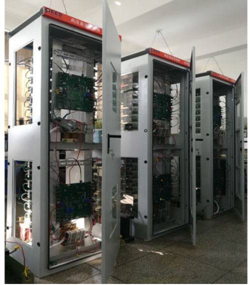
Fig. 5. Photograph of the laboratory three-phase MMC prototype.
