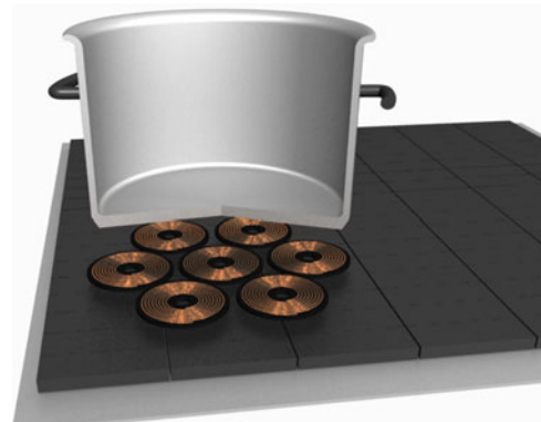
Fig. 1. IH coils with different electromagnetic coupling ratio to the IH target.
