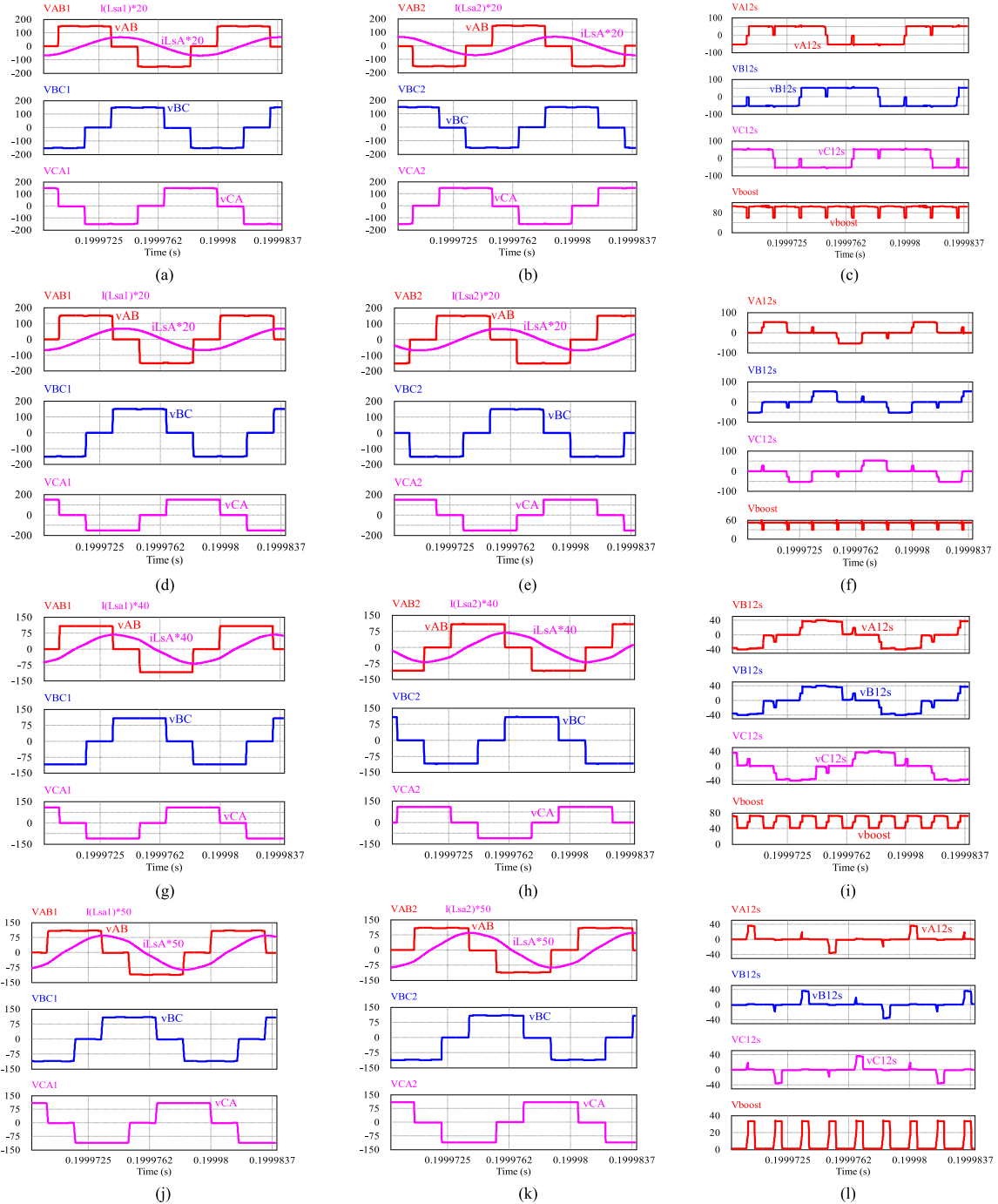
Fig. 9. PSIM simulation waveforms of the voltage across inverter output terminals ( v_{AB} , v_{BC} , v_{CA} ) and the current through phase A of the tank circuit ( i_{LsA} ) for: (a) module-1 and (b) module-2, and (c) the phase voltages across the secondary terminals of the 3-phase boost transformer T_3 ( v_{A12s} , v_{B12s} , v_{C12s} ), and the output voltage of the boost rectifier before filtering ( v_{boost} ); for case-1: V_{in}(\min) = 50 V, full-load, R_L = 60 \Omega , \delta = 180^\circ . Waveforms of (a)–(c) repeated: (d)–(f) for case-2: V_{in}(\max) = 100 V, full-load, R_L = 60 \Omega , \delta = 61^\circ , (g)–(i) for case-3: V_{in}(\min) = 50 V, half-load, R_L = 120 \Omega , \delta = 97^\circ ; and (j)–(l) Case-4: V_{in}(\max) = 100 V; half-load, R_L = 120 \Omega ; and \delta = 18^\circ .
