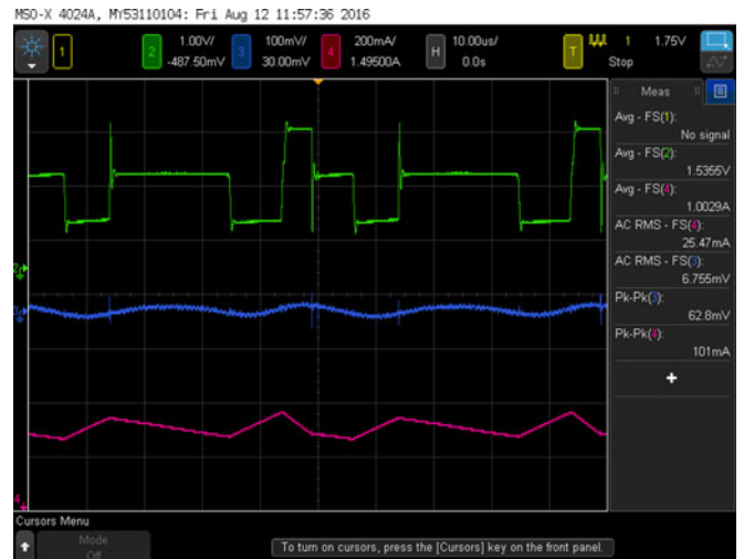
Fig. 9. Oscilloscope screen shot of the three smart cells operating at their optimal switching pattern, averaging applied with eight samples. Channel 2, top green trace, is the voltage across L_{sc} of the first smart cell with a capacity of C_1 . Channel 2, middle blue trace, is the output voltage ripple. Channel 3, bottom pink trace, is the current in the smart cell inductors.
