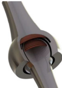
Fig. 4. View of the structure of the ball-joint WPT system with parts of the ball and ball-socket structures removed to show the embedded windings.
