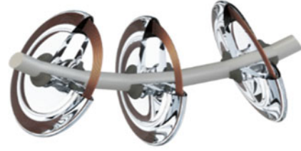
Fig. 3. Schematic of a “novel flexible insulation string” consisting of novel discs (with a section of the toughed glass removed to show the embedded copper coil of the resonator).
