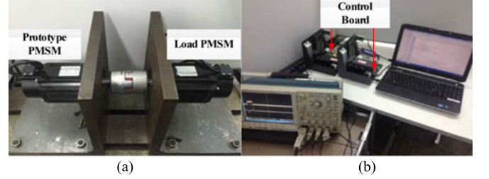
Fig. 6. Experimental platform of 750 W PMSM drive. (a) Load test platform. (b) PMSM driver system.
