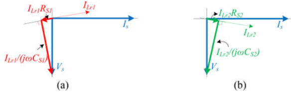
Fig. 18. (a) Phase diagram of V_s , I_s , and I_{Lr1} . (b) Phase diagram of V_s , I_s , and I_{Lr1} .
