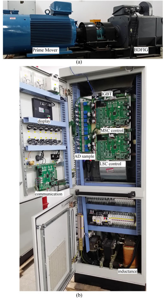
Fig. 10. Configuration of the experimental setup: (a) Prime mover and BDFIG system and (b) control system of the stand-alone BDFIG.
