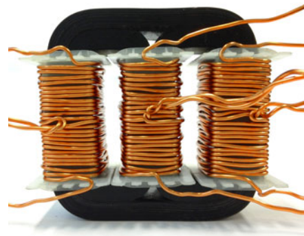
Fig. 10. Proposed inductor prototype; dimension of core: 80 \times 82 mm.
