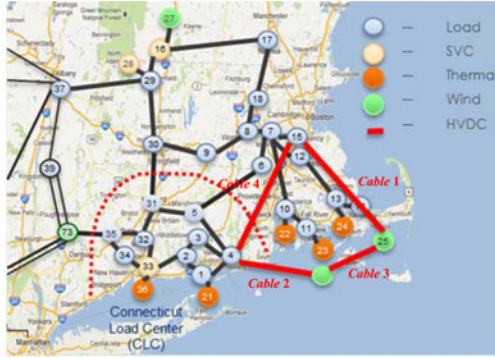
Fig. 2. Proposed hypothetical system corresponding to Cape Wind Project in Northeast Power Coordinating Council system.
