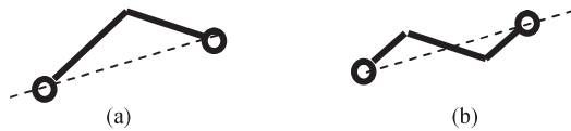
Fig. 8. Current (or flux) ripple shown in complex plane for (a) the previous single-ended SVM and (b) the novel state distribution (each trajectory direction corresponds to an active vector, V1 or V2 in example).
