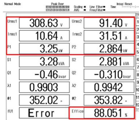
Fig. 20. Closed-loop system maximum power transfer capability test. ( U_{rms1} , I_{rms1} , and P_1 are the system input dc voltage, current, and power; U_{rms2} , I_{rms2} , and P_2 are the SC terminal voltage, charging current, and transferred power; Effice is the system efficiency).
