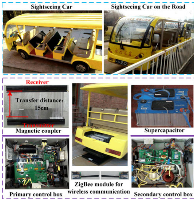
Fig. 15. Experimental setup of the WPT system.
