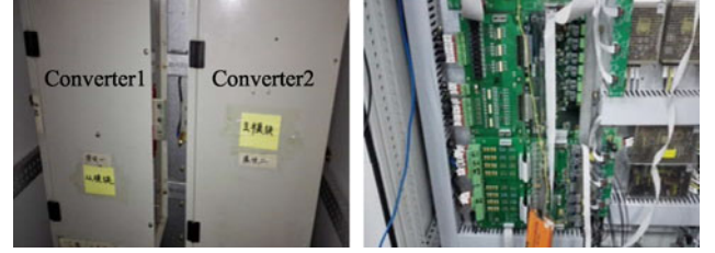
Fig. 11. Structure of parallel system. (a) Paralleled converters and filter inductance. (b) TMS320f2812 DSP based control board.
