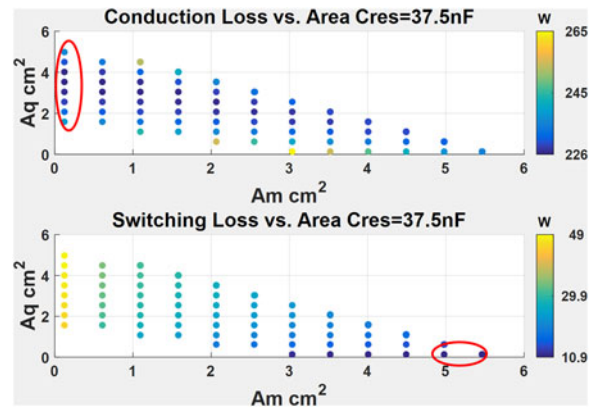
Fig. 15. Conduction loss versus switching loss ( C_{res} = 37.5 nF).
