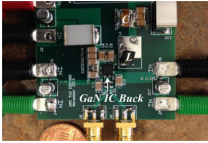
Fig. 22. Synchronous buck converter prototype with the GaN chip using the modified active pull-up driver.
