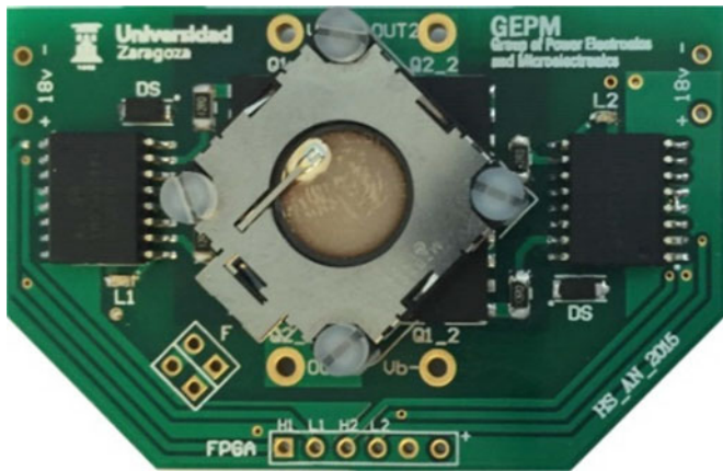
Fig. 18. Ultrahigh efficiency converter using piezoelectric thermal management: 600 W and 3.5-cm \times 5.5-cm PCB.
