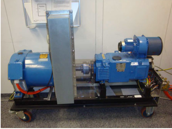
Fig. 8. Motor configuration at the test bed with the synchronous machine and a dc machine used as load.
