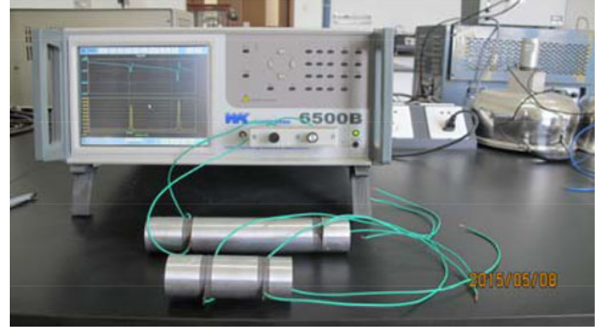
Fig. 15. Photograph of the frequency measurement setup of a wireless power transmission system.
