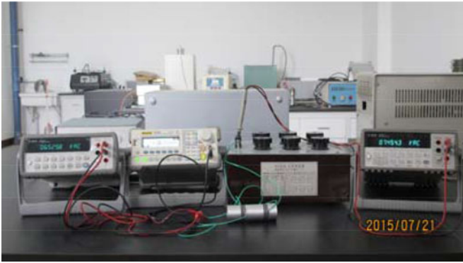
Fig. 16. Experimental setup for the measurement of the voltage gain.
