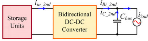
Fig. 3. Simplified configuration of the standalone photovoltaic power system when analyzing the SHC alone.
