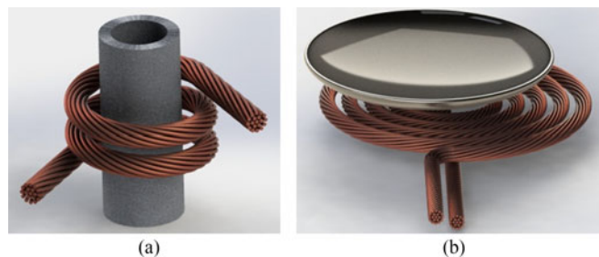
Fig. 1. Typical induction heating arrangements. (a) Planar. (b) Solenoidal.
