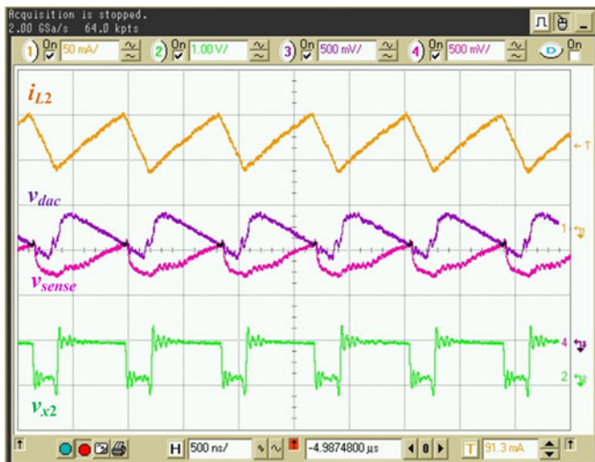
Fig. 34. Closed-loop CPM controller waveforms from MSC-DB implementation utilizing PMIC-BBs; Ch1: Inductor current, i_{L2} (50 mA/div); Ch2: switching node, v_{x2} (1 V/div); Ch3: DAC output with slope compensator (500 mV/div); and Ch4: senseFET output (500 mV/div).
