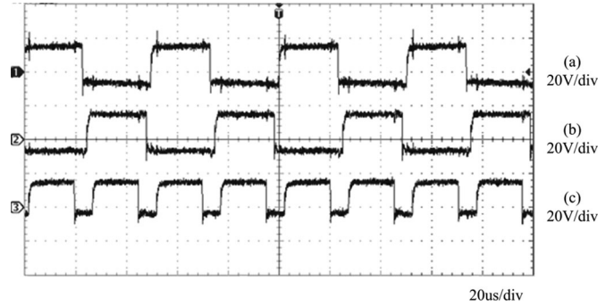
Fig. 6. Experimental results for the gate signals of power electronic devices, (a) gate signal of S_1 , (b) gate signal of S_2 , (c) gate signal of S_3 .
