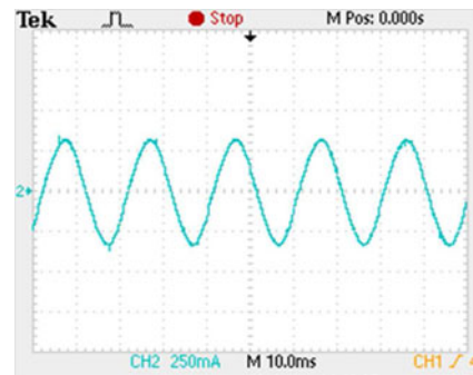
Fig. 20. Line current of prototype result for MI = 1 (CH1:10 ms/div, 250 mA/div).
