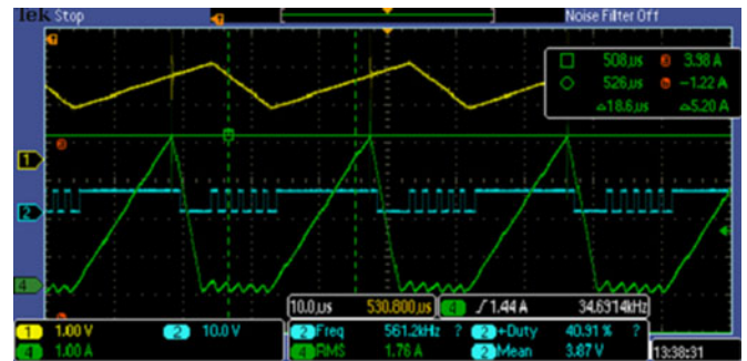
Fig. 14. Inverter waveforms at a dc operating point. Ch1 (yellow) cycle-by-cycle integration capacitor voltage v_{int}(t) , Ch2 (blue) auxiliary winding voltage sensor, at comparator output, Ch4 (green) inductor current i_L(t) . Conditions: V_{dc} = 426.8 V, I_{dc} = 0.98 A, v_{out} = 330.1 V, and i_{out} = 1.259 A.
