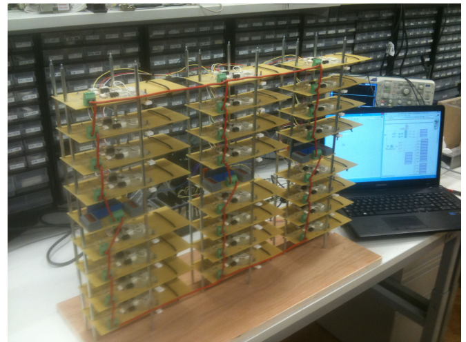
Fig. 11. Prototype of a five-level MMC with embedded lithium-ion batteries.
