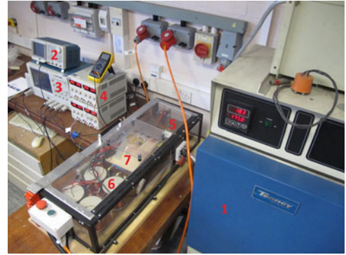
Fig. 2. Experimental setup. 1. The environmental chamber where the device temperature can be changed between -75 °C to 175 °C. 2. Function generator to produce double pulse. 3. Oscilloscope. 4. DC power supply for the gate drive and gate input signal. 5. DC link capacitors. 6. Inductive load. 7. Gate drive circuit.
