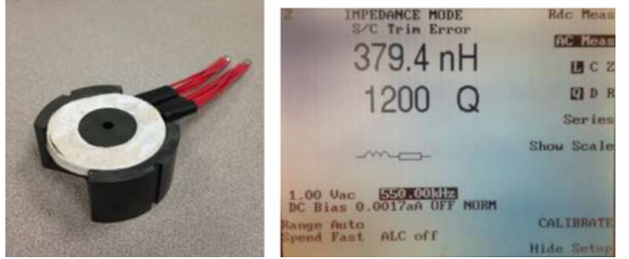
Fig. 6. Photograph of the prototyped high-Q resonant coil with a measured Q of 1200 at the resonant frequency of 550 kHz.
