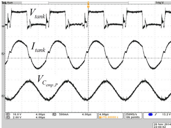
Fig. 11. Measured voltage waveforms across the resonant tank (upper trace, 10 V/div), compensating capacitor (lower trace, 2 V/div) and the current waveforms (middle trace, 500 mA/div) through the resonant tank at time scale of 4 \mu s/div.
