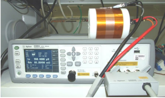
Fig. 10. Test setup for inductance measurement.
