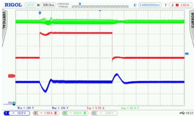
(b) Top: input voltage (10V/div), Middle: output current (1.5A/div), Bottom: output voltage (10V/div), Time: 500 \mu s/div.
