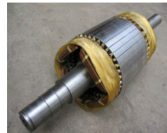
Fig. 6. Prototype rotor winding structure.
