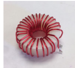
Fig. 6. Wire-wound counterpart inductor for comparison with the PCB inductor in Fig. 4. The dimensions are listed in Table III.
