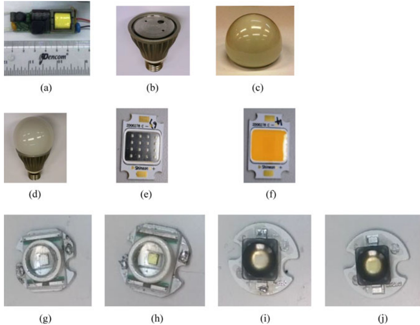
Fig. 4. Photographs of the exterior and interior functional stages of an LED bulb. (a) Ballast. (b) Heatsink. (c) Cover/lens. (d) LED bulb. (e) Shineon blue LED. (f) Shineon white LED. (g) Cree-XRE Blue LED. (h) Cree-XRE white LED. (i) Osram-W5AP Blue LED. (j) Osram-W5AP white LED.
