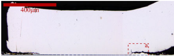
Fig. 13. Optical microscopy image of a wire/IGBT interface on section 3 of module C.
