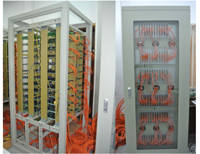
Fig. 9. Photo of the single-phase MMC prototype.
