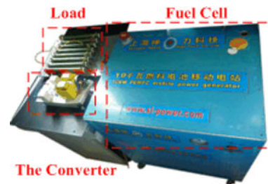
Fig. 11. Prototype of the 1-kW Converter with fuel cell and load.
