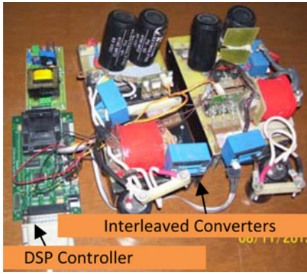
Fig. 14. Experimental setup: compensation converters along with TMS320F2812 controller.
