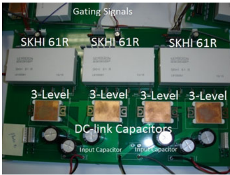
Fig. 8. Single phase of a nine-level cascade converter.
